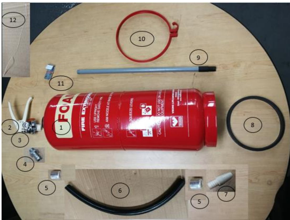
Figure 1: Dismantled 6kg Powder Cartridge Operated Fire Extinguisher
